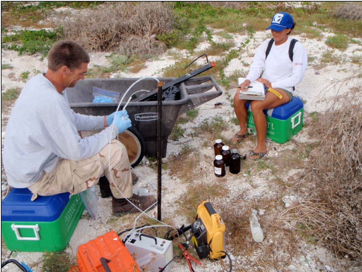
Collection of groundwater sample from peizometer using peristaltic pump.
