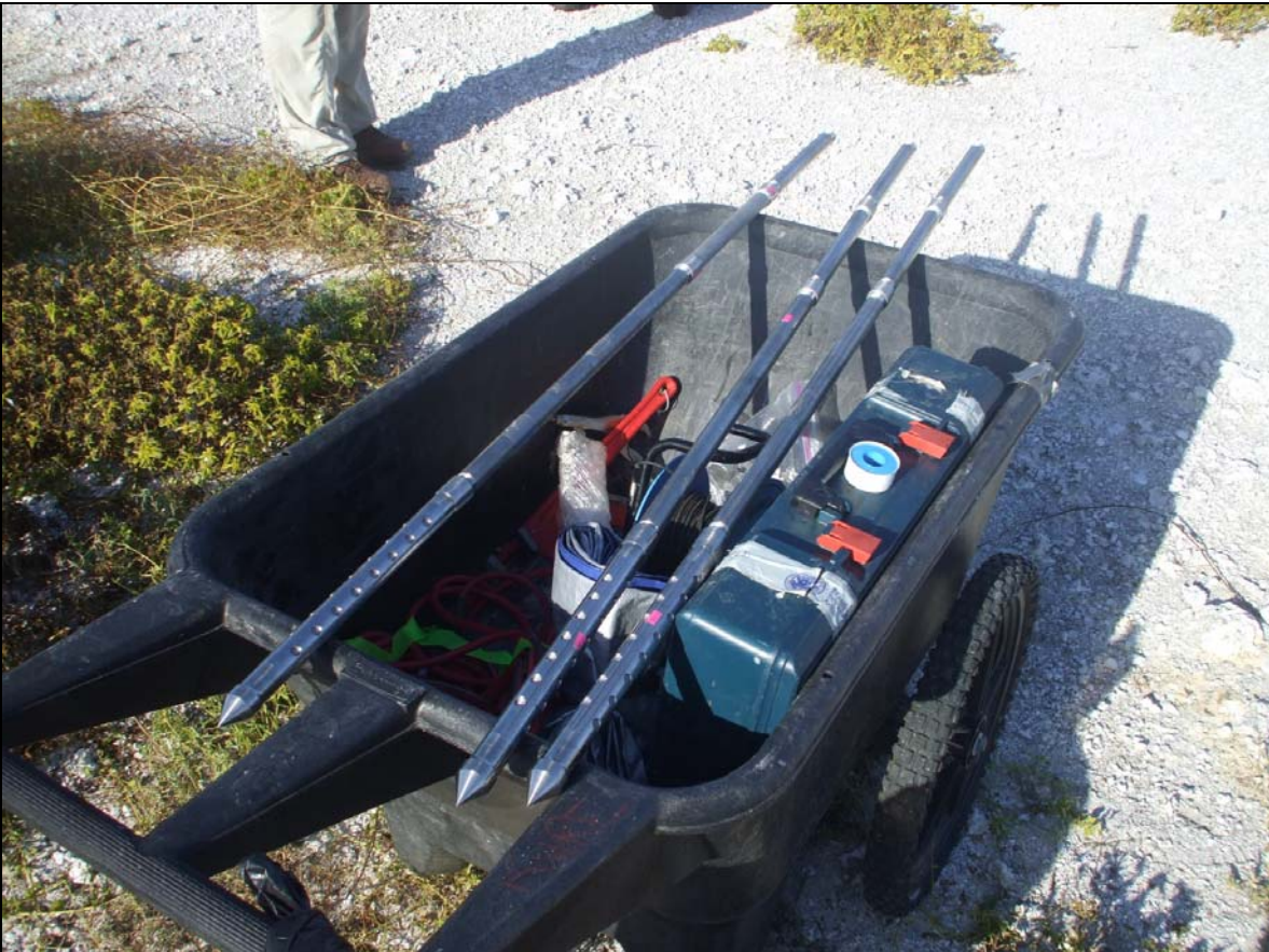
Piezometers prior to decon and installation.
