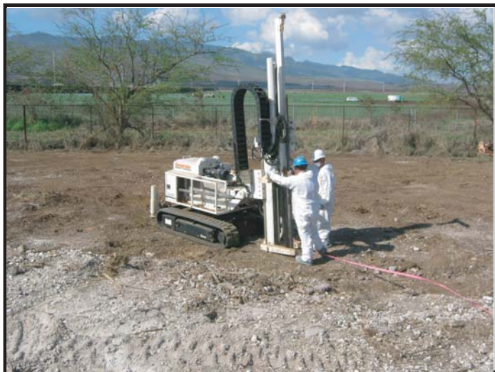
Photo 5: View of Geoprobe direct-push rig operation
