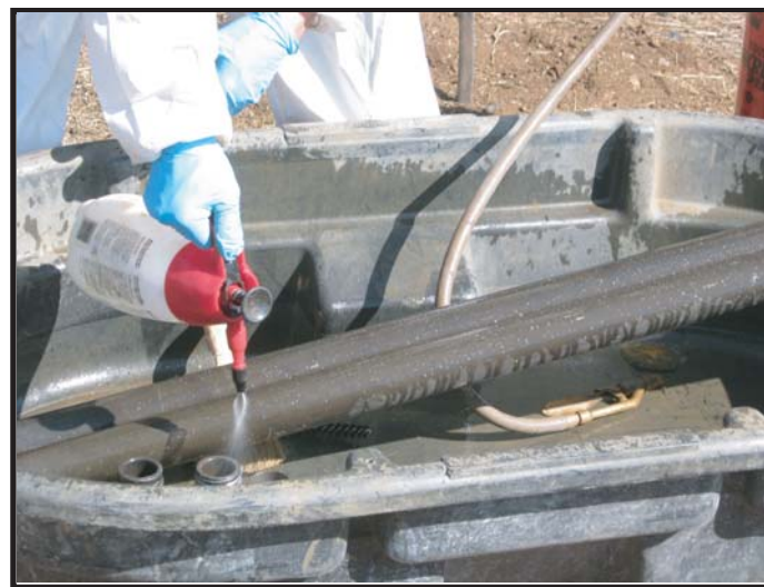
Photo 8: Typical view of core sampler decontamination
