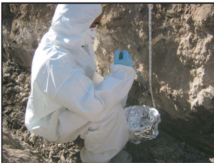
Photo 11: ETC personnel collecting soil increment from trench
