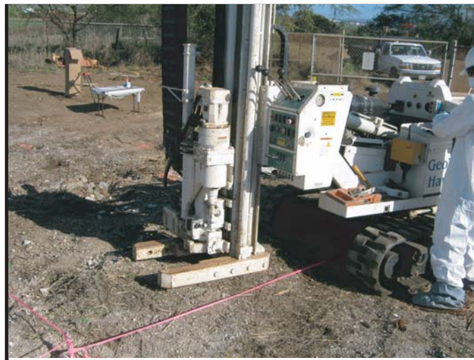
Photo 6: collection of soil boring from Spill Area
