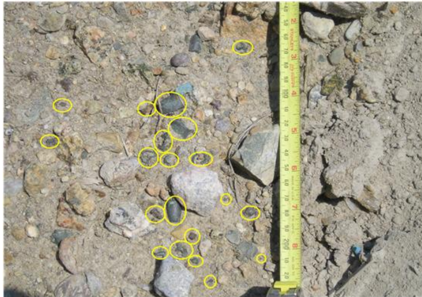
Figure 1. Visible small-arms metal debris (yellow circles) found on a small-arms range at Camp Edwards, Massachusetts.
