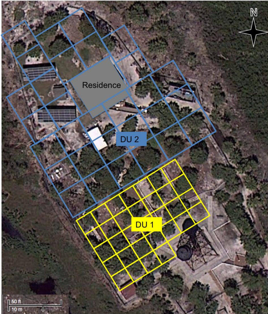
Figure 2. Schematic representation of the sampling grids for DU1 and DU2. Anclote Key Lighthouse, Pinellas County, Florida. Figure was modified from aerial map of Anclote Key Preserve State Park obtained from Google maps ( http://maps.google.com/ ).
