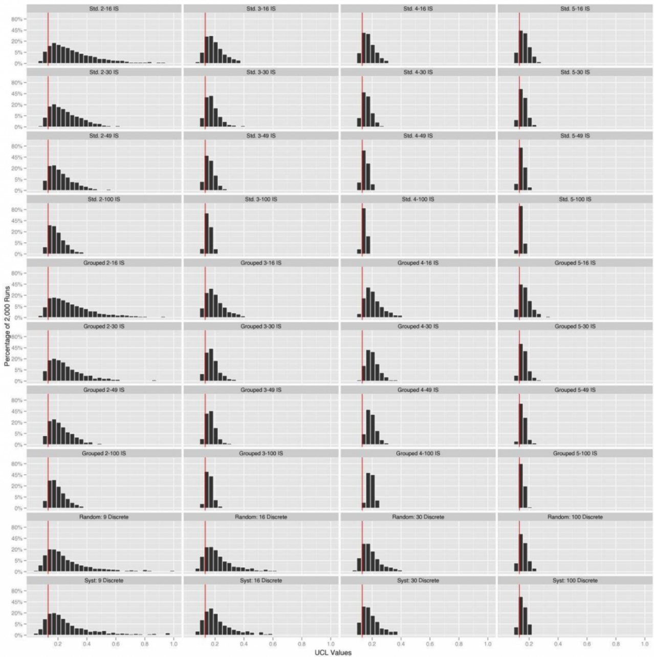
Figure B-15. Panel of histograms of the distribution of 95% t-UCL values for the 2,000 simulations. Note that the red line identifies the true mean. The y-axis identifies the percent of 2,000 simulations in each bin and is distorted to show the percentage in the low count bins.
