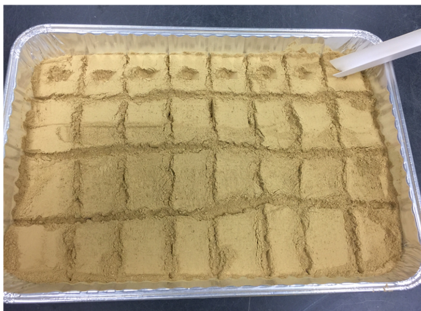
Figure 5-8. Two-dimensional slabcake with square scoop.
