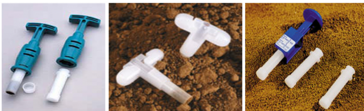
Figure 5-10. Examples of coring devices for VOC soil increment collection. Core N' One™ tool (left), Terra Core Sampler (center), and Easy Draw Syringe® and PowerStop Handle® (right). 2020.
