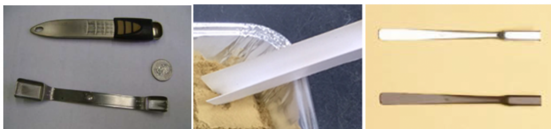
Figure 5-9. Examples of rectangular and flat-bottom sampling tools.
