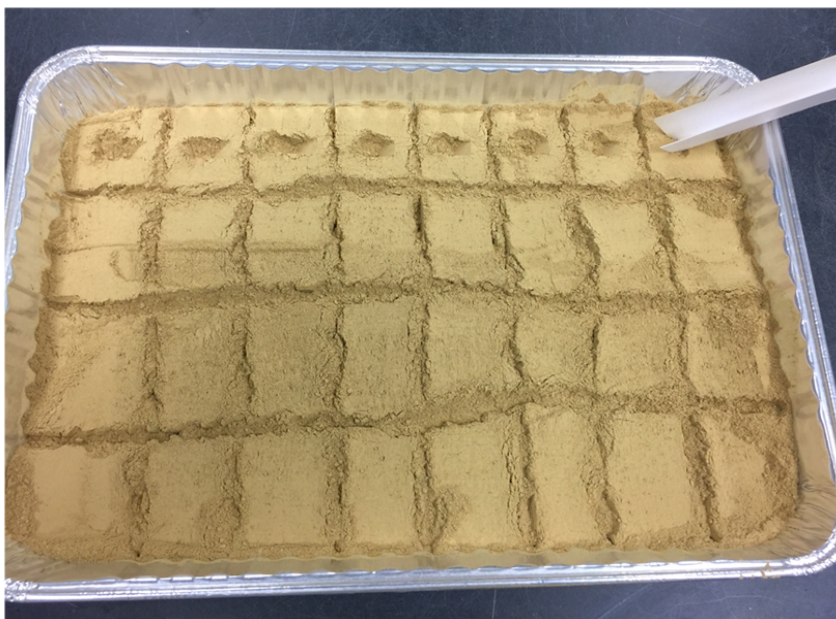
Figure 5-8. Two-dimensional slabcake with square scoop.
