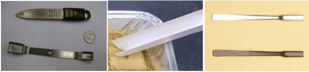
Figure 5-9. Examples of rectangular and flat-bottom sampling tools.
