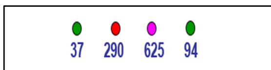
Figure 2-9. Arsenic concentrations for in situ XRF readings spaced about 2 ft apart in a residential yard.
